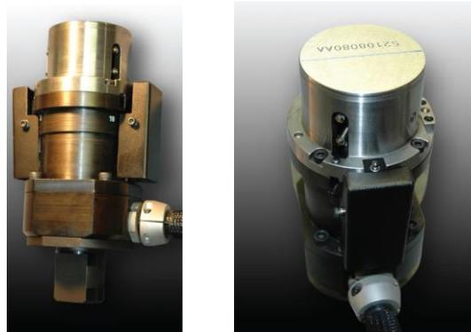
Figure 14. A specially developed, sensor supported, mechanical gage unit for shop-floor inspection of gears (Baruchello, R and Sicheneder, G, 2009)
