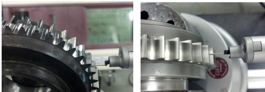
Figure 11. MDP ground gear (left) and conventionally ground gear (right) (DeAngelo, J A. 2017)
