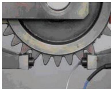
Figure 1. Single tooth bending fatigue test rig (Gasparini et al 2009)
