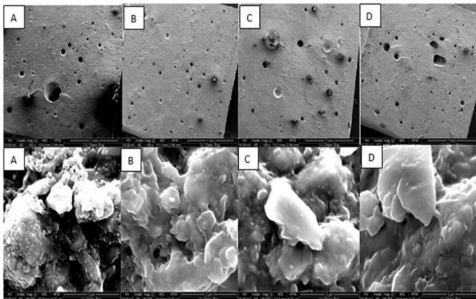
**Figure 2:** The fractured surfaces of BAG modified compomer restorative materials, SEM images. A: %1 BAG, X1.000, A: %1 BAG, X60.000, B: %2 BAG, X1.000, B: %2 BAG, X60.000, C: %3 BAG, X1.000, C: %3 BAG, X60.000, D: %4 BAG, X1.000, D: %4 BAG, X60.000.
