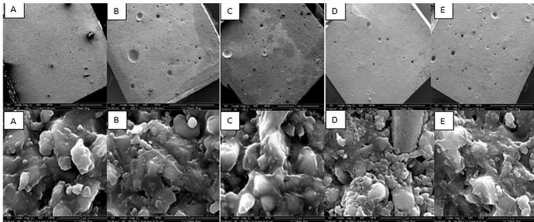
**Figure 1:** The fractured surfaces of HA modified compomer restorative materials, SEM images. A: Control, X1.000, A: Control, X60.000, B: %1 HA, X1.000, B: %1 HA, X60.000, C: %2 HA, X1.000, C: %2 HA, X60.000, D: %3 HA, X1.000, D: %3 HA, X60.000, E: %4 HA, X1.000, E: %4 HA, X60.000.
