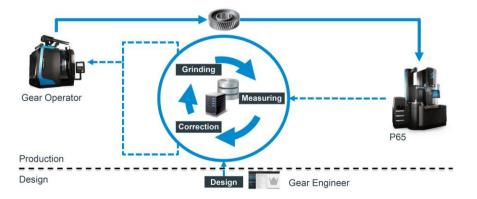
Figure 15. Closed Loop production system, Gear Engine (Brumm M and Müler, H., 2018)
