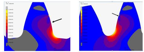
Figure 7. Symmetric and asymmetric root forms (Akpolat et al 2017)
