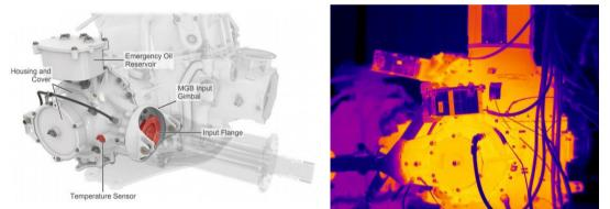
Figure 2. AW189 input module view and heat distribution on the AW189 MGB (Gasparini et al 2014)
