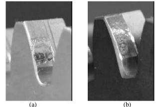
Figure 4. Typical appearance of failed gear tooth surfaces. (a) Uncoated gear. (b) Coated gear. (Krantz et al 2003)
