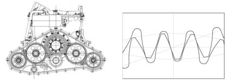
Figure 5. Main transmission combining gearbox section view and HCR gear teeth (Yıldırım et al 2008)
