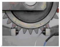
Figure 1.Single tooth bending fatigue test rig (Gasparini et al 2009)
