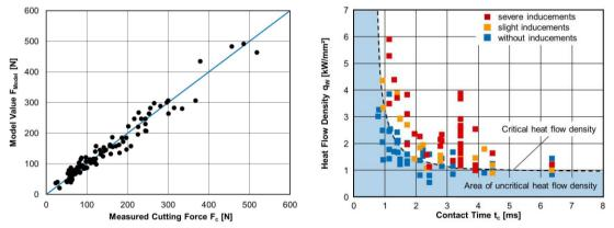
Figure 12. Grinding cutting force measurements and surface zone inducements depending on heat flow density (Ophey, M and Reimann, Dr. J, 2014)
