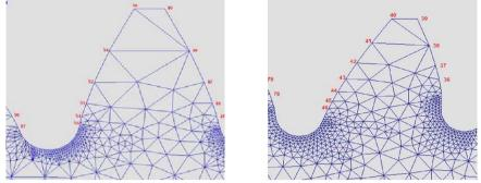
Figure 6. Symmetric and asymmetric tooth forms (Brown et al 2010)
