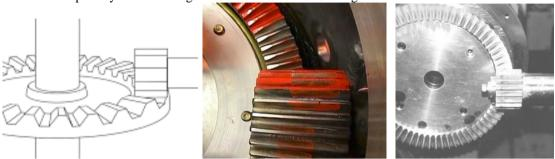
Figure 9. Face gears (Heath et al. 2002)
