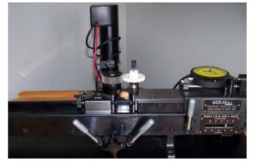
Figure 13. A double-flank composite tester in tight mesh
