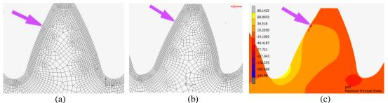
Figure 8. Symmetric tooth symmetric root (a), Asymmetric tooth asymmetric root (b,c) (Şahin et al 2018)
