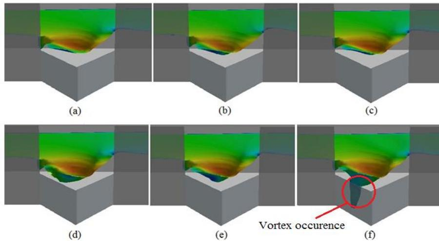
Fig.2. Vortex occurrence in a triangular labyrinth side weir for different turbulence models: a) Spalart-Allmaras, b) k-omega, c) Standard k-epsilon, d) RNG k-epsilon, e) Realizable k-epsilon, f) RSM model (Aydin 2012)
