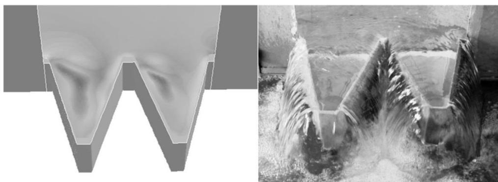
Fig. 4. Views of free surface flows over a labyrinth side weir: (a) CFD, (b) Experimental.
