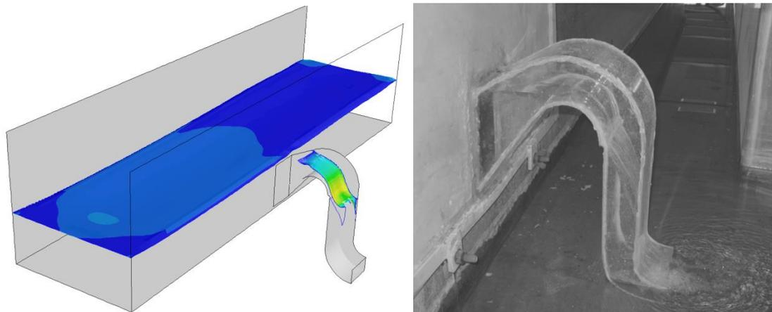
Fig 5. CFD simulation of a siphon side weir.
