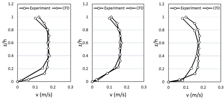
Fig. 6. Velocity profiles along flow depth at the main channel centerline (Aydin et al. 2015)
