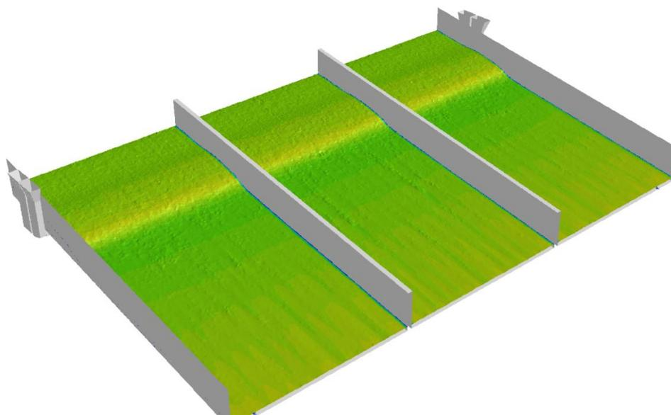
Fig. 7. CFD simulation of spillway aerator of a large dam (Ilisu Dam Spillway in Turkey).
