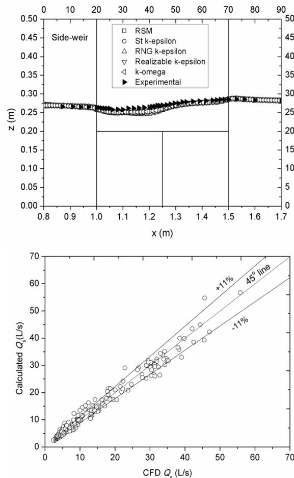
Fig. 1.a) Free surface levels over a triangular side weir for different turbulence models and experimental (Aydin 2012), b) Comparison discharges obtained by CFD with empirical results. (Aydin and Emiroglu 2013)
