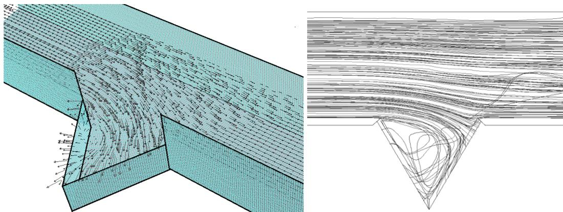
Fig 3. CFD views of side weir: velocity vectors and pathlines over the side weir flow.
