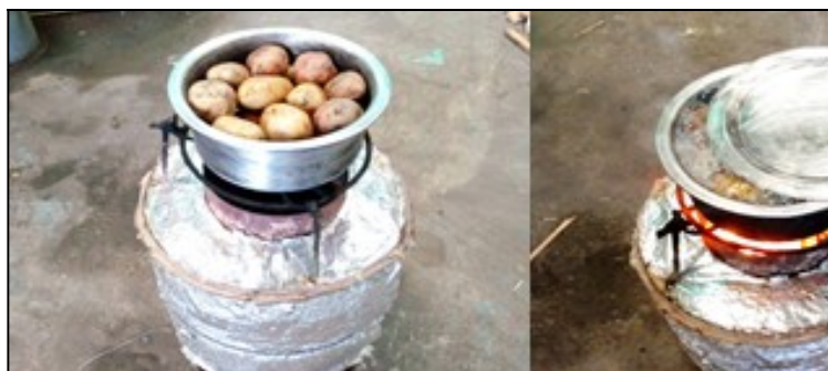
Fig.5 The wood gas cook stove test with insulator (glass wool)
