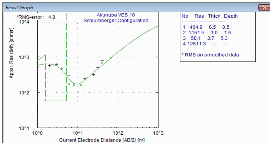
Figure 4 b: Typical KH Curve Type.
