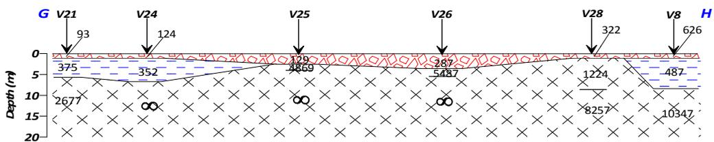
Figure 5 d: A NW-SE Geoelectric Section obtained along Line G-H (Resistivity values in  $\Omega m$ ).
