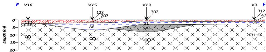
Figure 5 c: A NW-SE Geoelectric Section obtained along Line E-F (Resistivity values in  $\Omega m$ ).
