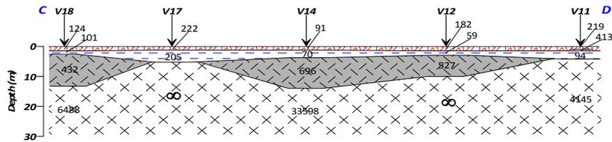
Figure 5 b: A NW-SE Geoelectric Section obtained along Line C-D (Resistivity values in  $\Omega m$ ).
