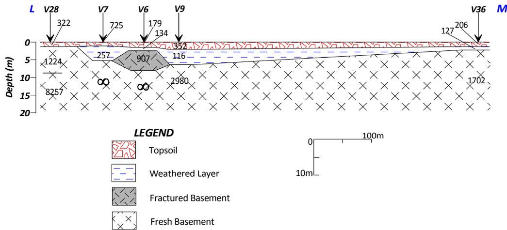
Figure 5 g: A SW-NE Geoelectric Section obtained along Line L-M (Resistivity values in  $\Omega\text{m}$ ).
