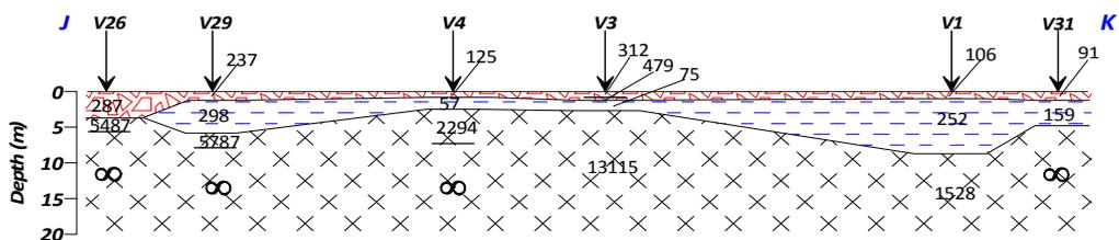
Figure 5 f: A SW-NE Geoelectric Section obtained along Line J-K (Resistivity values in  $\Omega m$ ).
