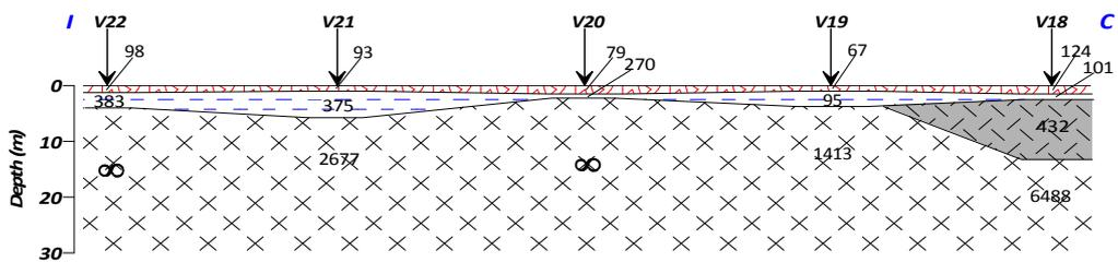
Figure 5 e: A SW-NE Geoelectric Section obtained along Line I-C (Resistivity values in  $\Omega m$ ).
