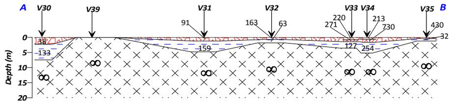
Figure 5 a: A NW-SE Geoelectric Section obtained along Line A-B (Resistivity values in  $\Omega m$ ).
