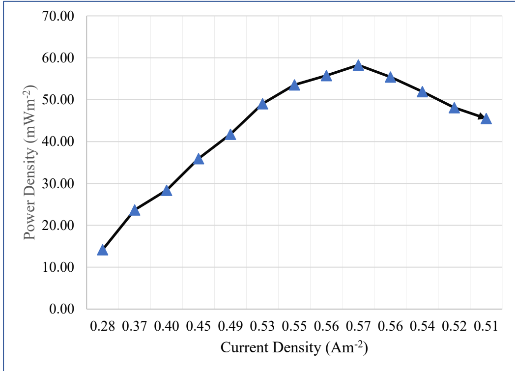
Fig. 4: The power density curve for reactor
