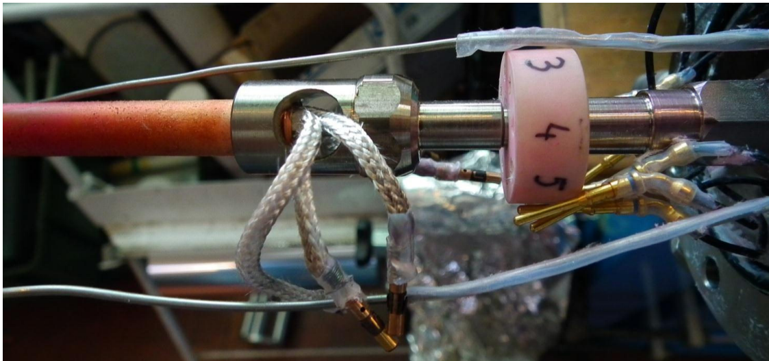
Figure 18. Real assembly: details of “head” with electrical feed-through, under assembling.
