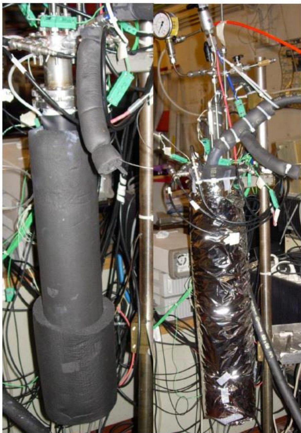
Figure 22. Real reactor: steps 6-7 of assembly, final thermal insulation.
