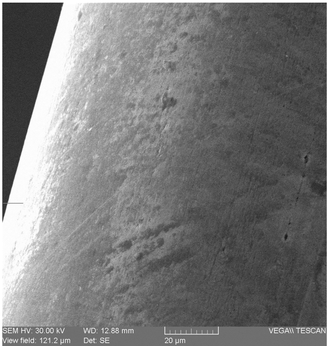
Figure 4. SEM. Details of wires after plastic removal: almost smooth surfaces.
